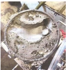
Example of Aluminum Sludge, dehydrated in 30sec. inside the unit
