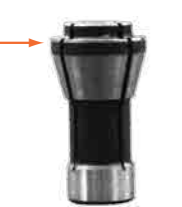
Standard Collet Grips at 1 location.
