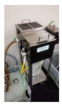
High performance two-stage separation mobile floating sludge collecting unit.
